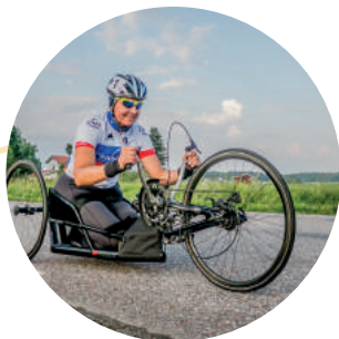
A paracycle that facilitate cycling for people with physical disabilities.
